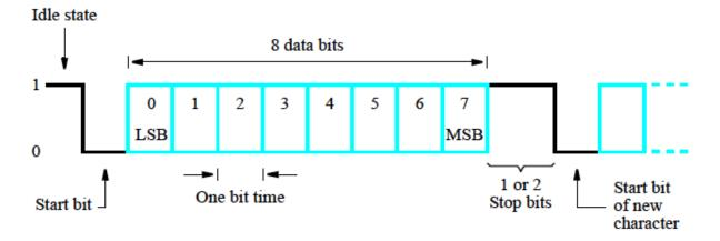
As seen in the lecture, using a "start-top" scheme with the Universal Asynchronous Receiver Transmitter (UART) requires the receiver's clock to run at *approximately* 16x the speed of the transmitter clock to transfer 8 bits of information correctly.
